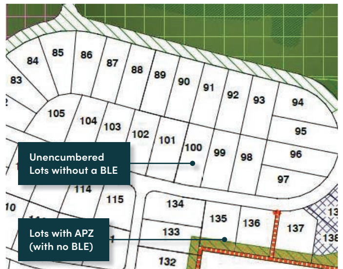
Figure 3 - Example of lots without a BLE that are either completely unencumbered or have APZ on them (Source: Approved Park Lake Adare Conservation & Building Location Envelope Plan).
