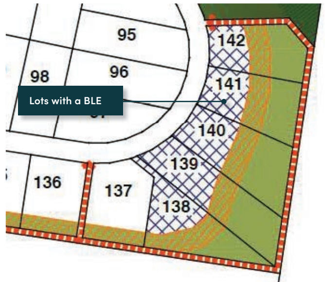
Figure 2 - Example of Lots with BLEs on private land with APZ and Conservation Areas. (Source: Approved Park Lake Adare Conservation & Building Location Envelope Plan).
